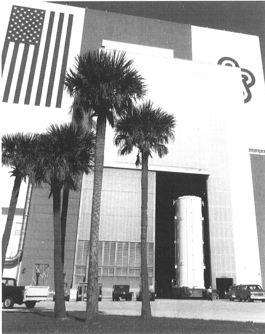
Figure 4. Payload canister exiting the Vehicle Assembly Building (VAB), undated. (Courtesy of Kennedy Space Center, Image 108-KSC-80P-367.jpg).
