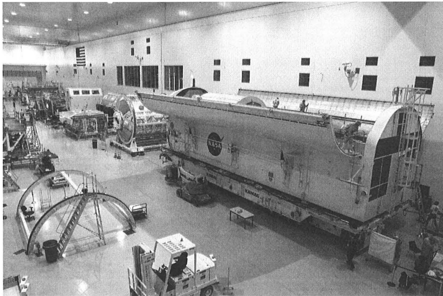
Figure 22B. Canister's doors open in the SSPF. October 21, 2008. (Courtesy of Kennedy Space Center, KSC-08PD-3300 10_21_08.jpg).
